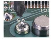
Camout and tool/recess wear can also create damaging debris. This diminishes the aesthetic value of the fastener, and, more importantly, can cause irreparable damage in electronic assemblies, airbags, and other critical applications.
