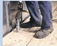
Difficulty in aligning the drive bit and the recess can force an assembly line to slow down to assure proper fastening.
